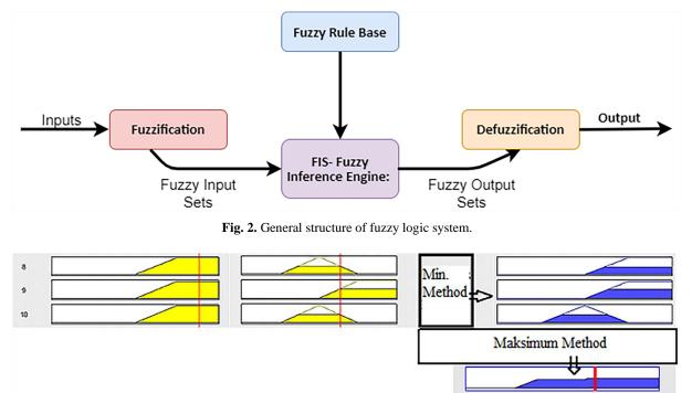
Fig. 3. A fuzzy system using the minimum (min) method for firing rules and using the largest (maximum) method for the combining process.
