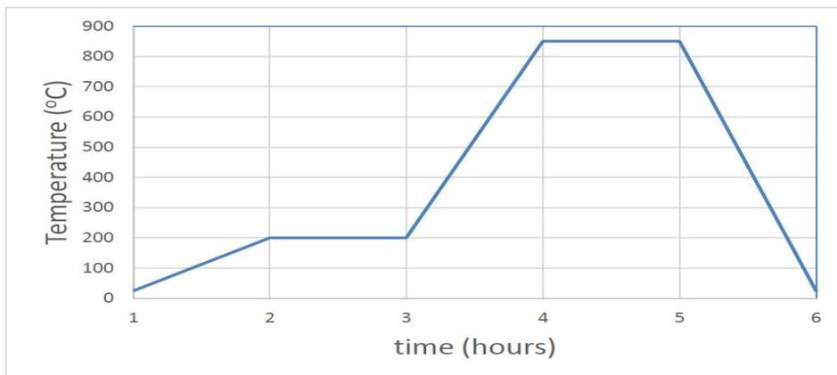
**Figure 4.** Sintering Temperature-Time
