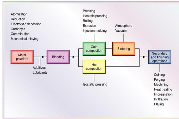
**Figure 3.** The powder metallurgy production method flow chart
