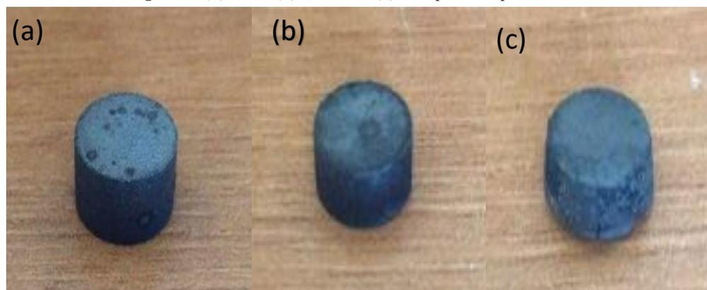
*Figure 6. (a) 50%, (b) 70% and (c) 80% porous specimens*
