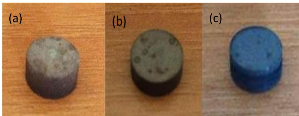
*Figure 5. (a) 20%, (b)30% and (c)40% porous specimens*
