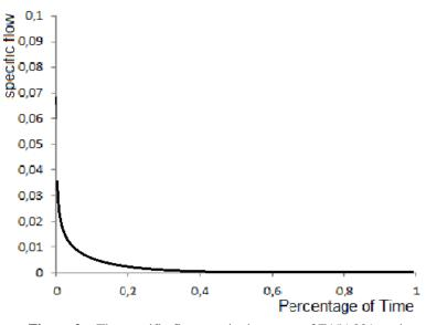
Figure 2a. The specific flow continuity curve of E15A001 station.
