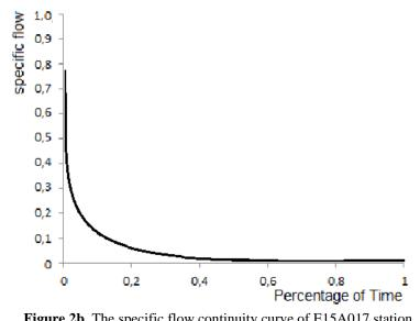
Figure 2b. The specific flow continuity curve of E15A017 station.
