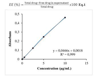
Figure 1. Calibration curve of ceftiofur.
