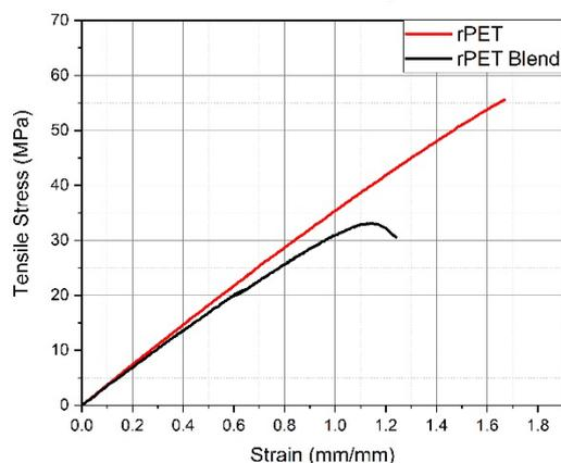
**Figure 6.** The representative stress-strain curves of tension test.
