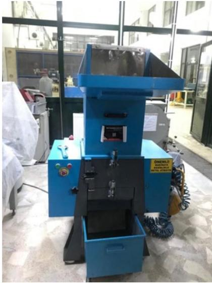
Figure 2. Blade mill shredder.
