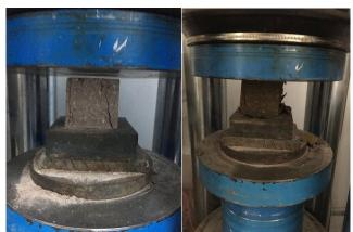
Figure 1. The compressive strength test of the samples
