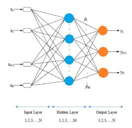
Figure. 1. Single-Hidden layer feed forward network architecture
