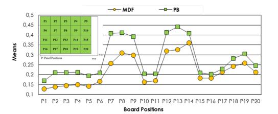
The differences between the FE values according to the different positions of the MDFs were tested with ANOVA. In the analysis results in Table 6, prominent differences between the variables including the measurement results of the FE in the different board positions were determined to be statistically important at a level of p < 0.001 level for all the items (1st, 2nd and 3rd hours) related to the scale.
